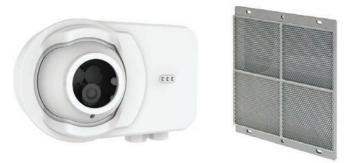
The OSI-R is a reflector- type linear optical beam smoke detector designed to operate as a component of fire alarm systems. The beam operates primarily on the principle of light obscuration utilising an Infra-Red beam. Optical beam smoke detectors are particularly appropriate for protecting buildings with large open spaces such as warehouses, atriums etc.
